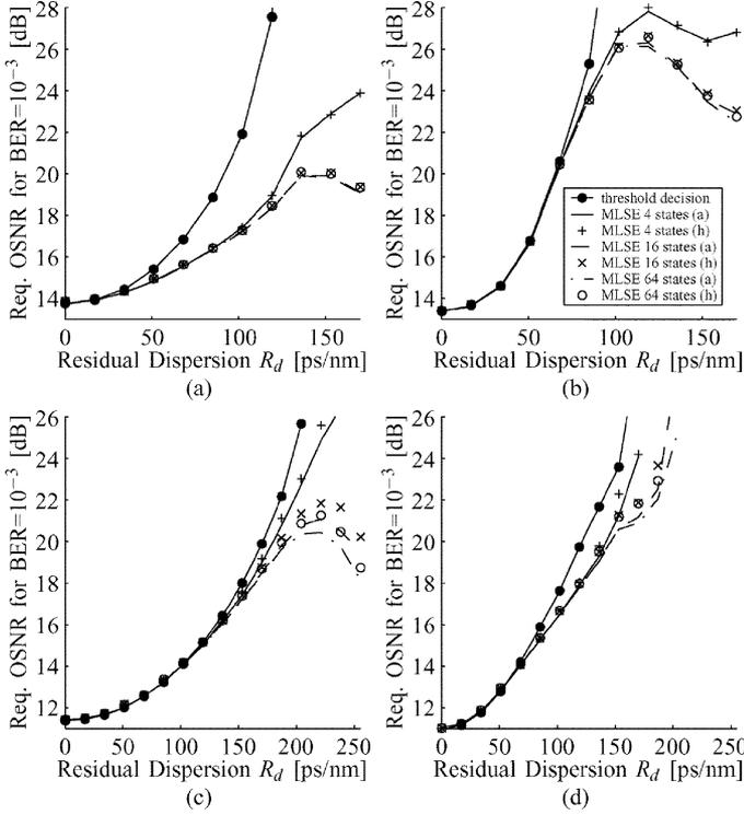
Fig. 4. Required OSNR for  $\text{BER} = 10^{-3}$  versus residual dispersion for (a) NRZ-ASK, (b) RZ-ASK, (c) NRZ-DBPSK, and (d) RZ-DBPSK.
