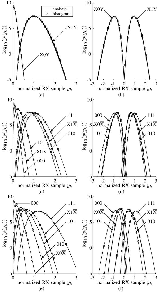
Fig. 2. PDF for (a) ASK and (b) DBPSK at  $R_d = 0$  ps/nm. (c) ASK and (d) DBPSK at  $R_d = 85$  ps/nm. (e) ASK and (f) DBPSK at  $R_d = 170$  ps/nm.
