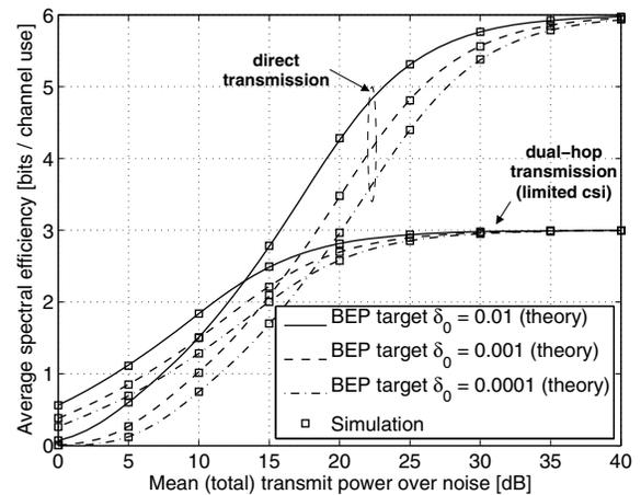
Fig. 3. Average spectral efficiency as a function of the mean (total) transmit power over noise. In case of dual-hop transmission, the per-hop BEP targets are set to  $\delta_1 = \delta_2 = \delta_0/2$  and a path loss exponent of  $\nu = 4$  is assumed.
