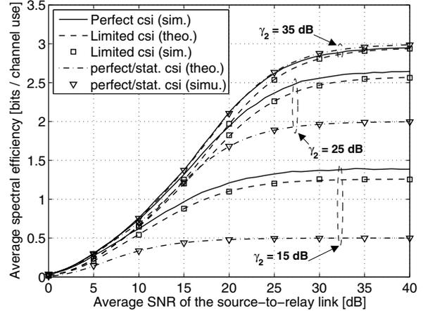
Fig. 1. Average spectral efficiency versus the average SNR on the source-to-relay link for an end-to-end BER target of  $\delta_0 = 10^{-2}$ . In case of adaptation based on limited csi, the per-hop BER targets are set to  $\delta_1 = \delta_2 = 0.005$ .
