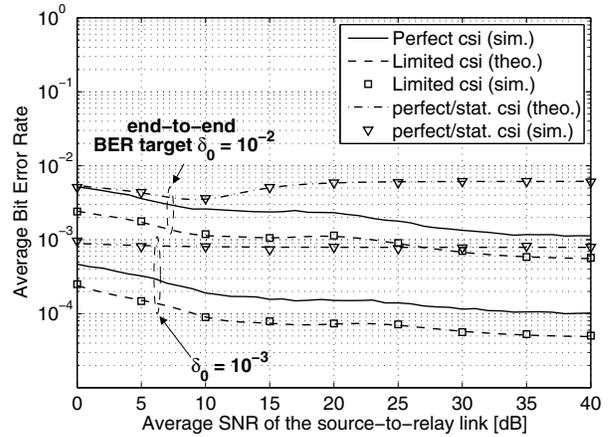
Fig. 2. Average end-to-end BER as a function of the average SNR on the source-to-relay link for  $\delta_1 = \delta_2 = \delta_0/2$  and an average SNR on the relay-to-destination link of  $\bar{\gamma}_2 = 25$  dB.
