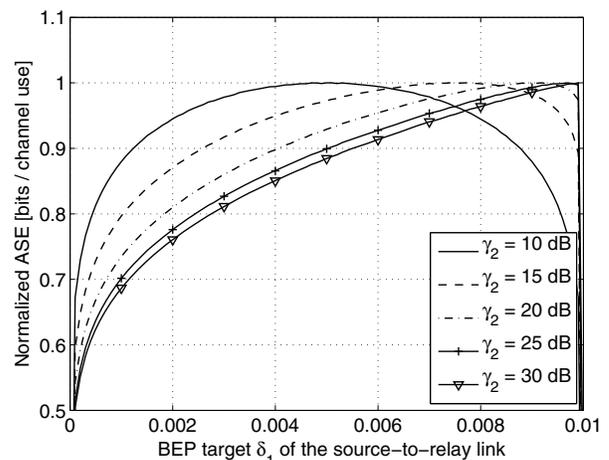
Fig. 4. Average spectral efficiency normalized to the respective maximum value versus the BEP target  $\delta_1$  on the source-to-relay link for  $\bar{\gamma}_1 = 10$  dB,  $\delta_0 = 0.01$ , and different average SNRs of the relay-to-destination link.
