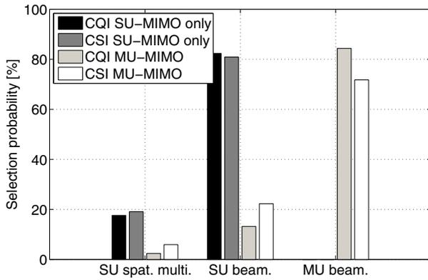
Fig. 5. Transmission scheme selection probabilities of various cases for the Macro 1 case.
