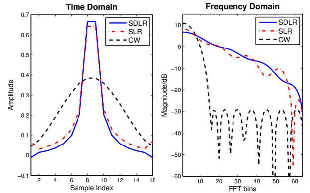
Fig. 3: Filter, optimized for timing and frequency offset in the range of  $\pm 5\%$  in time and frequency domain
