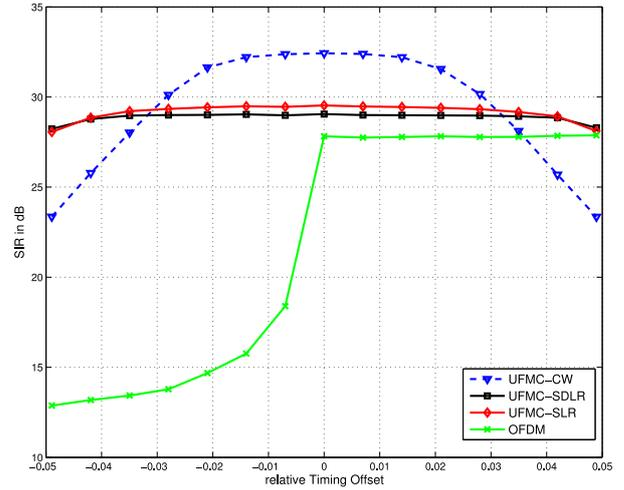
Fig. 2: SIR Comparison for different system settings under rCFO  $\epsilon = 0.05$
