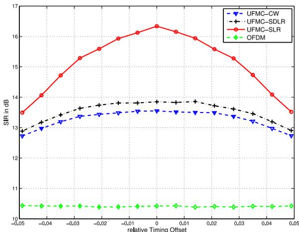
Fig. 4: SIR Comparison for different system settings under rCFO  $\epsilon = 0.5$
