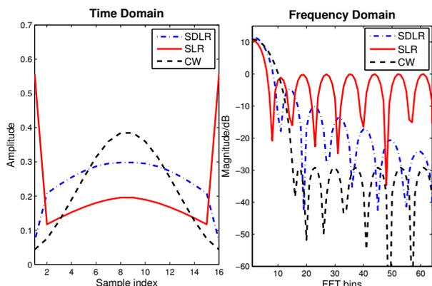
Fig. 5: Filter, optimized for timing offset range of  $\pm 5\%$  and rCFO range of  $\pm 50\%$  in time and frequency domain
